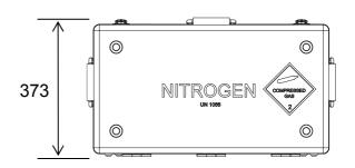
Additional handles are fitted to allow for two-man lifting.
