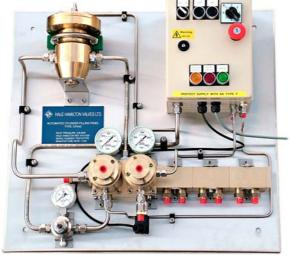
Our customer fills breathing air cylinders for use in fire fighting. The existing method of filling was to use a stop valve to blast air into the cylinders as fast as possible. This process created excess heat during the filling process and resulted in a settled pressure far below the required 276 barg.
